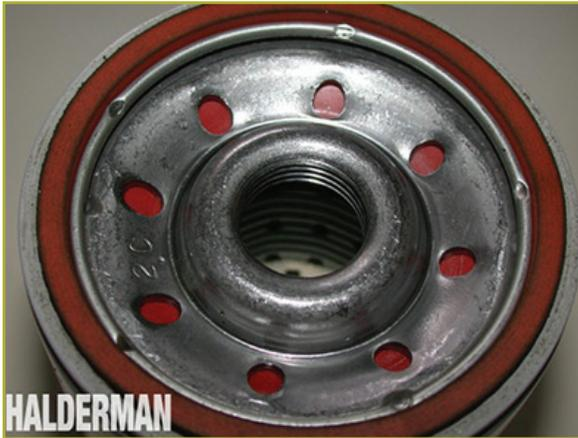
**FIGURE 14— Spin-On Filter Gasket**
