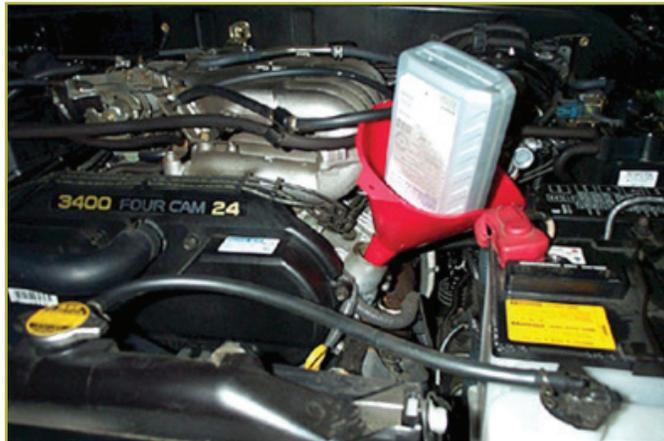
Start the engine and observe the oil pressure warning light. It should go out within a few seconds once the engine is running. If the light doesn't go out, shut the engine down immediately and tell your supervisor or instructor. If the light goes out, shut off the engine and recheck the engine oil level. Some of the oil goes in the filter, and the level may drop slightly. The level with a full filter should be at the full mark or slightly below the mark. Top off as needed.
