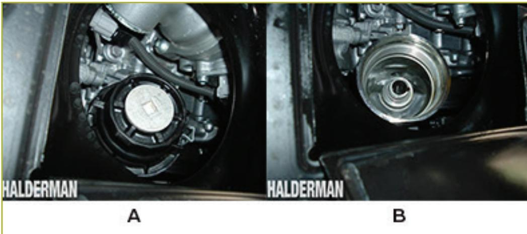
**FIGURE 11—Cartridge Oil Filter with Top (A) and Without (B)** (Courtesy of James Halderman)
