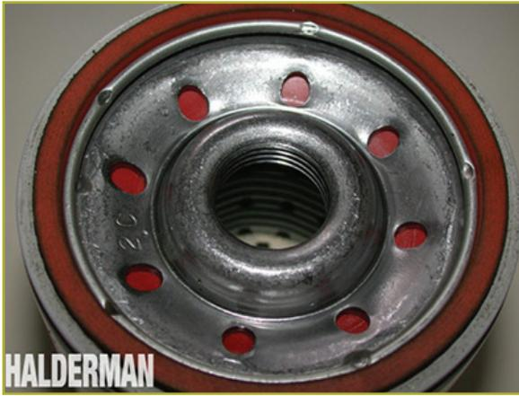
**FIGURE 14— Spin-On Filter Gasket**
