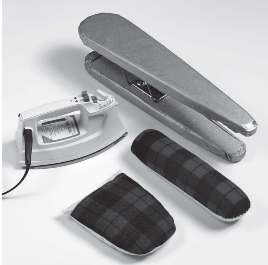
FIGURE 1 —Pressing equipment (L to R, iron, pressing cushion, seam roll, sleeve board)
