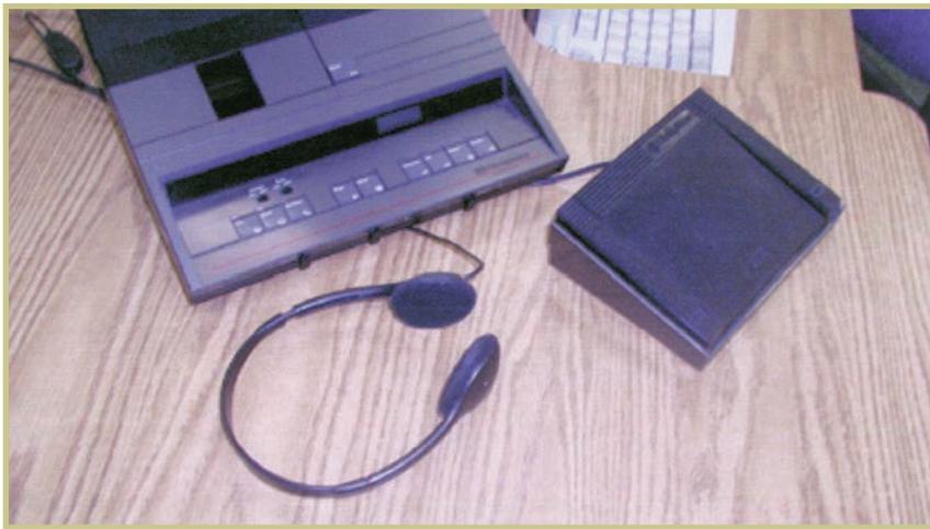
FIGURE 4—Desktop Transcription System with Foot Pedal
